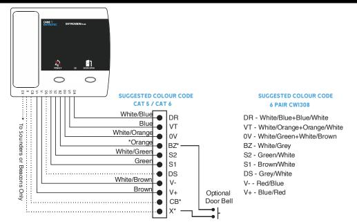
\* NOTE: If DS is required the internal ringer can be enabled and the BZ connection is not required, freeing up the Orange wire.
